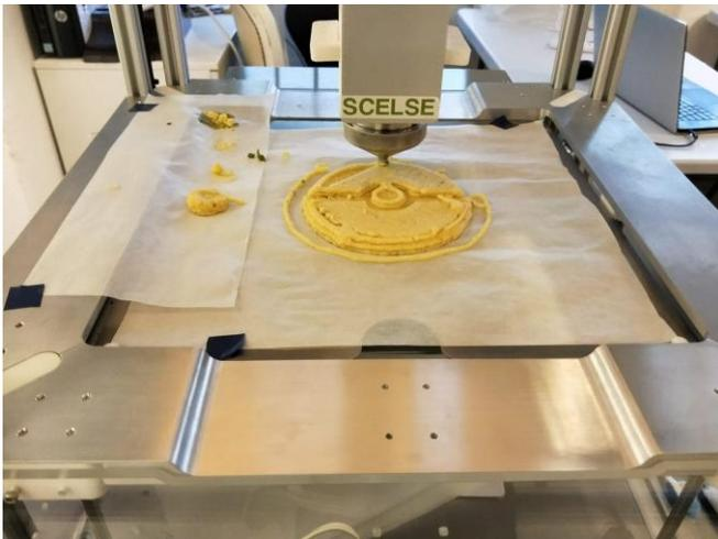
*Anrich3D uses extruders to deposit layers of food paste in three dimensions.*
